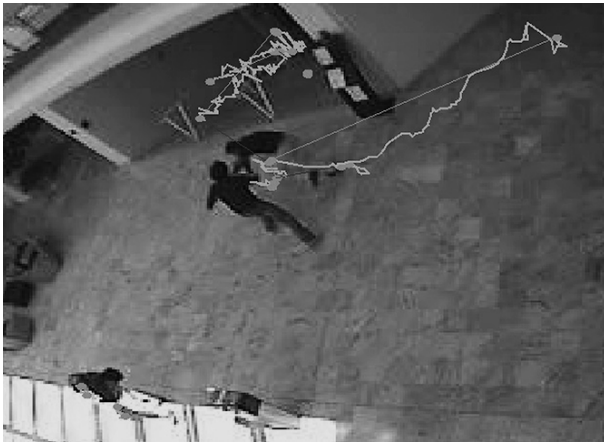
Fig. 1. A situation like a street incident (fight between two people) comes into the field of view of the intelligent video surveillance program. Heavy solid lines show the trajectories of people, and thin lines and circles indicate connected graphs of motions of blobs.
