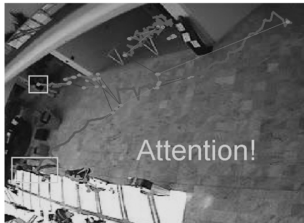
Fig. 2. The intelligent video surveillance program has recognized a situation like a street incident. Heavy solid lines show the trajectories of people involved in a probable street conflict, thin lines and circles indicate connected graphs of motions of blobs, and rectangles represent the people involved in the incident.
