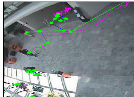
Figure 3: A low-level procedure discriminates trajectories (violet lines) of objects and moments of their interactions (green circle marks and blue links).
