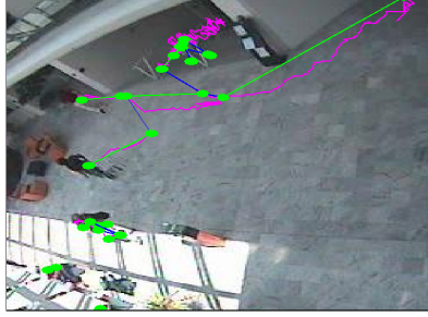
Fig. 3. A low-level procedure discriminates trajectories (violet lines) of objects and moments of their interactions (green circle marks and blue links).
