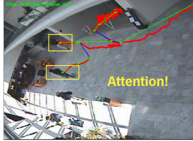
Fig. 5. A logical inference has found a possible case of a sudden attack in the graph of blob trajectories. Rectangle blobs are depicted by yellow lines, blob trajectories are depicted by red lines, moments of interactions between blobs are depicted by green circles and blue links.
